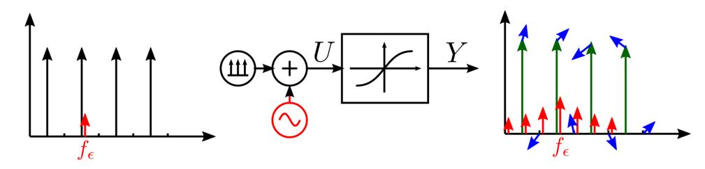
$$Y(f_k) = U(f_k) \cdot \left( G^{[1]}(f_k) + \sum_{i=-N}^{N} G^{[3]}(f_i, -f_i, f_k) \cdot |U(f_i)|^2 + \sum_{i=-N}^{N} \sum_{j=-N}^{N} G^{[3]}(f_i, f_j, f_k) \cdot U(f_i)U(f_j) \right)$$
