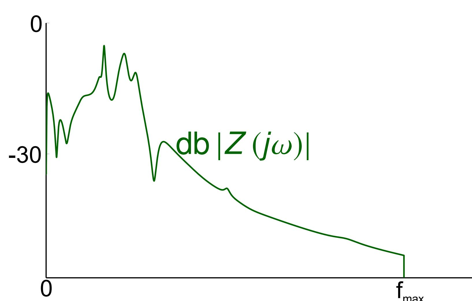
Circuit contains delay  $\Rightarrow Z(j\omega)$  is non-rational
