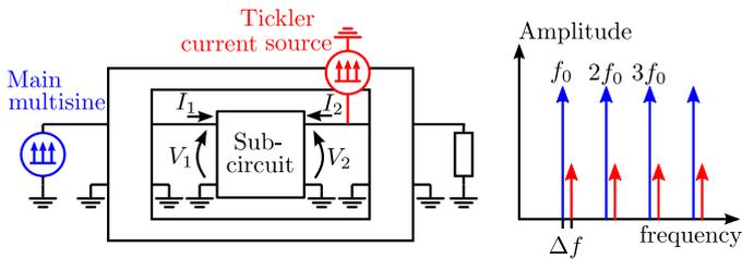
Figure 3. Estimating the BLA of a sub-circuit requires extra tickler multisines (red) around the sub-circuit. Placing the ticklers on a frequency grid with a small offset  $\Delta f$  allows to obtain the response of the tickler without influence from the main multisine.
