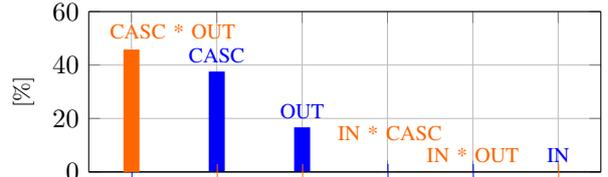
Figure 6. The DCA finds that the dominant source of distortion is the cascode stage. The strong correlation with the output stage (shown in orange) indicates that the distortion is generated at the interface between both stages. All other parts contribute for less than 1% to the total distortion.
