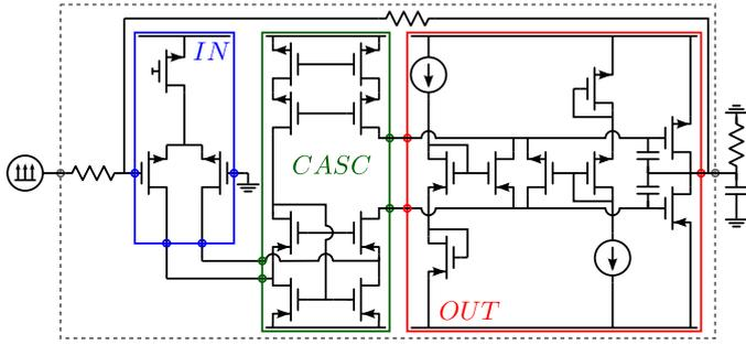
Figure 5. Push-pull op-amp used as an example. The op-amp is placed in an inverting feedback configuration with a gain of 5. The load consists of a 10pF capacitance and a 1k $\Omega$  resistor.
