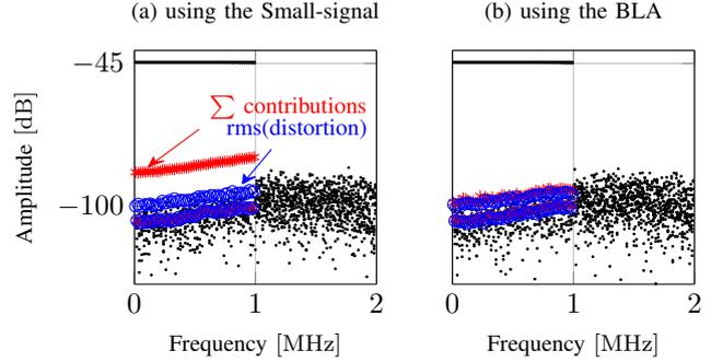
Figure 7. Using the small-signal behaviour of the circuits in the DCA leads to a large error (a). With the new estimation algorithm for the BLA, the error is removed (b). The steady-state spectra for the different realisations of the multisine are shown in black, The sum of the contributions (+) should match the rms of the circuit distortion (o).
