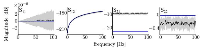
Figure 4. Using an extra tickler multisine at the output of the class-C amplifier allows to determine the MIMO BLA of the transistor. The BLA and its  $3\sigma$  uncertainty bound are shown in black. The small-signal S-parameters are shown in blue.
