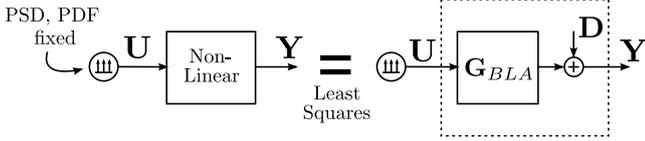
Figure 1. The response of a non-linear system to a fixed class of input signals can be approximated by a linear response. The residual is the distortion introduced by the system.
